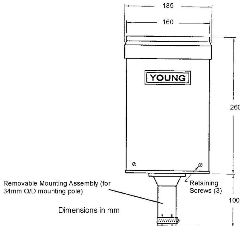
Figure 1 Dimensions of 52202/52203 Tipping Bucket Rain gauge
