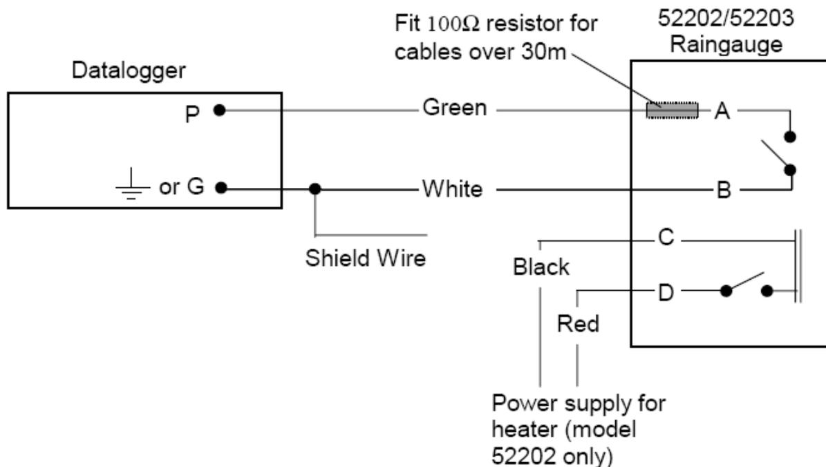
Figure 2 Wiring Diagram for 52202/52203
